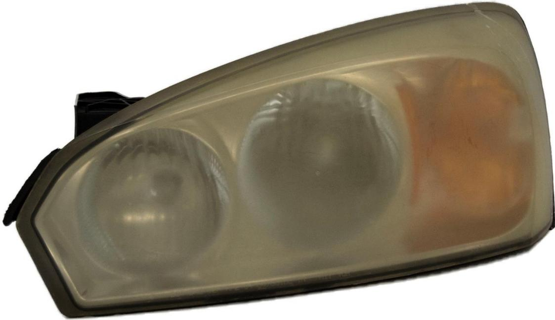
Figure 32: Malibu Used 2 Deteriorated
