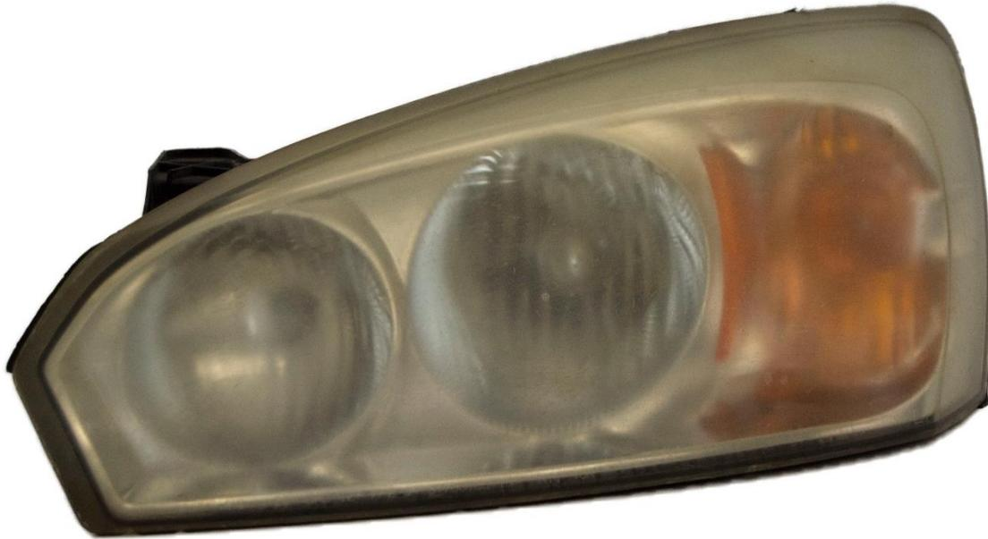
Figure 30: Malibu Used 1 – Deteriorated
