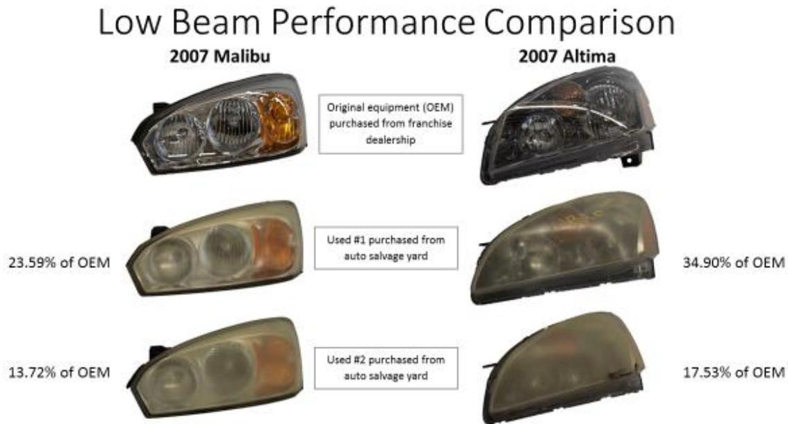
Figure 6: Low Beam Illumination Performance Comparison
