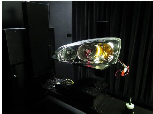
Figure 2: Chevy Malibu headlamp mounted on goniophotometer
