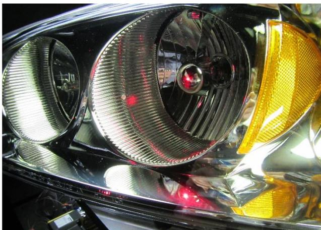
Figure 3: Laser aimed at headlamp for initial alignment
