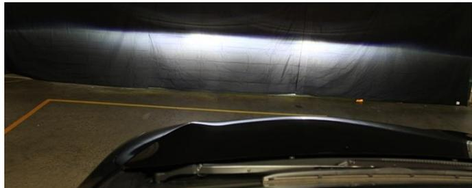
Figure 4: Low beam headlamp pattern showing horizontal cutoff
