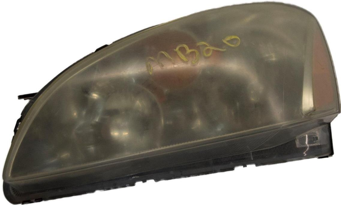
Figure 34: Altima Used 1 Deteriorated
